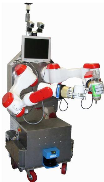
**Figure 1.** The TAMS service robot TASER as research object for our high-level episodic robot memory system.
